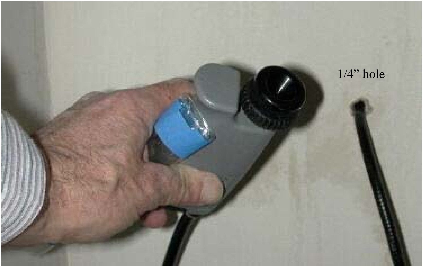
BORESCOPE - Used to inspect inside walls
